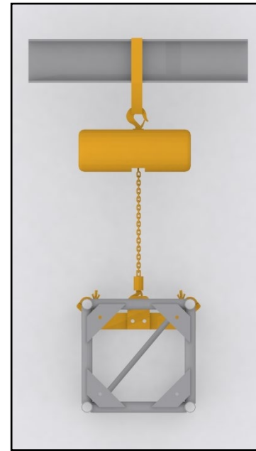
Fig. 20 - Dynamic Load Path (12.3.6)
