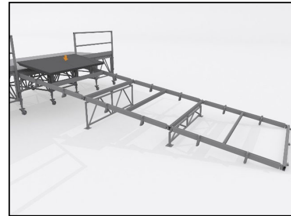
Fig. 50 – Fit the Special Top Deck
