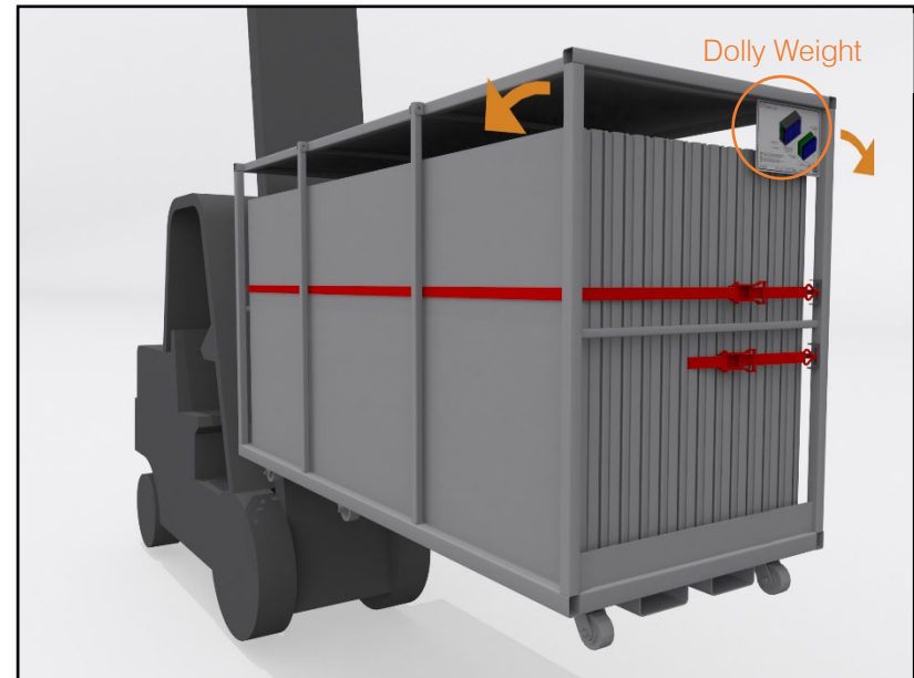
Fig. 67 – Balanced Load to stop overturning during handling
