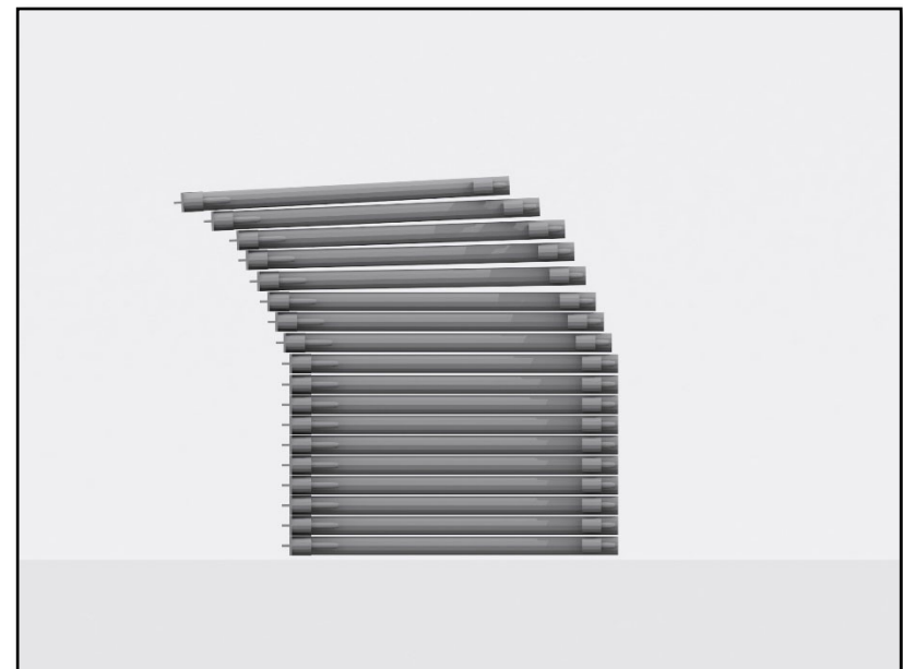
Fig. 66 – Unstable stacking of Components
