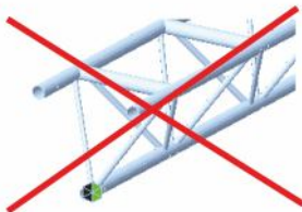
Figure 3: Not allowed orientation of the truss supported of bottom chords
