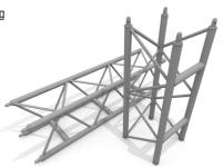
The OV range is a series of square and triangular truss systems using conical connectors for a quick fixing method. Brace patterns are specifically designed to withstand the loads and forces implied by all common slinging and support methods. The extrusions used in the construction of the trusses are bespoke to Total Solutions Group and have been rigorously designed to enhance the structural effectiveness of the trusses and also to speed up manufacturing.
